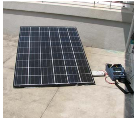
Fig. 2 Experimental setup for solar module under testing
